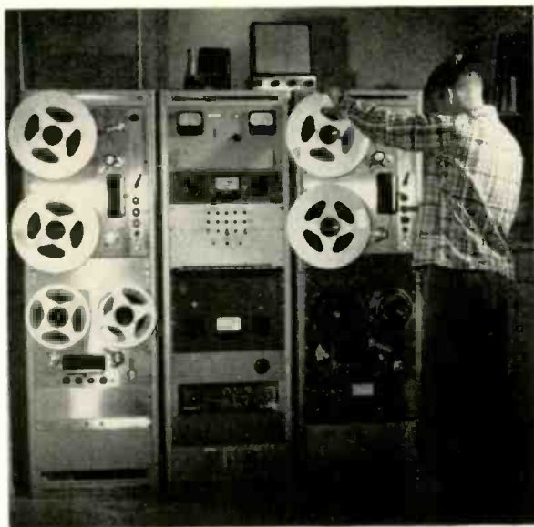
Unique to FM broadcasting is this automated tape system supplied, with recorded programs, by International Good Music, Inc. System is built around modified Ampex units. Top decks play music; deck at lower left plays local commercials and announcements; remaining deck is a stand-by unit. Timing and switch controls are housed in center console.
