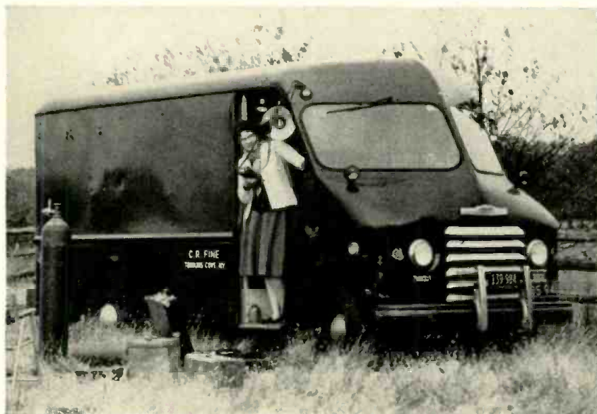
Miss Cozart directs the firing from Mercury's truck—a control room that houses two three-channel stereo tape recorders as well as two independent monophonic ones.
